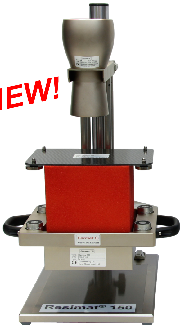
Figure 1: Mechanical set of Resimat 150 with the innovative ultrasonic fan-sensor LR 4 (top). It is designed to measure the recovery of a viscoelastic foam cube with 150mm edge length (red). Four software controlled clamps keep the sample down during the hold time.
