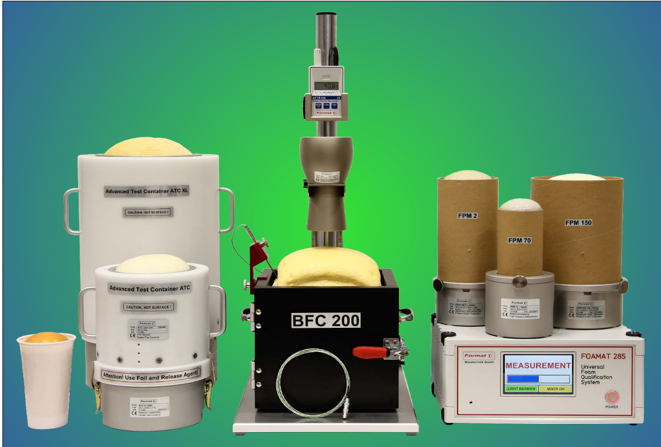
Figure 1: The Universal Foam Qualification System FOAMAT 285 is supplied with different test containers. The base system consists of the stand, the ultrasonic fan sensor LR 4 , the controller unit, and the PC software FOAM . The Advanced Test Containers ATC and ATC XL (left) are the most sophisticated test containers. The innovative Box Foam Container BFC 200 is used for slabstock foam. The Foam Pressure Measurement devices FPM 2 , FPM 70 and FPM 150 (right) use disposable cardboard cylinders of different diameters. Disposable cups can also be used. Patent Nos. 3621819, 19730891 and 10044952
