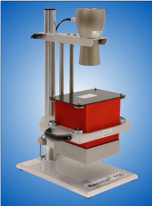
Figure 20: Resimat 150 is designed for the measurement of the recovery time of viscoelastic foams according to the IKEA ® specification IOS-MAT-0076 . The cubic test sample (red) has an edge length of 150 mm.
