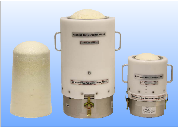
Figure 8: The Advanced Test Container ATC XL (center) has four times the test volume of the standard ATC (right). Each of them comprises an upper and a lower part, which are clamped by spring locks. The foam sample (left) can easily be ejected through the bottom opening of the upper part.
