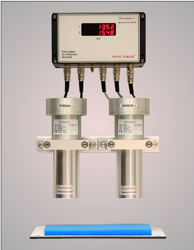
Figure 25: The Controller Unit SONIC JOKER and the two ultrasonic Fan-Sensors FS 2 are mounted for the thickness measurement of open celled foams, lying on a reference surface.
