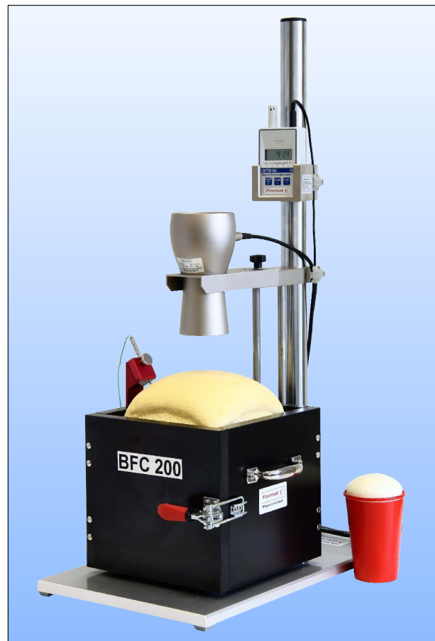
Figure 7: The BFC 200 (Box Foam Container) is placed onto the base plate of the stand. A thermocouple is inserted into the foam using a special positioning holder. The ambient data is measured by the meteorological station GFTB .
