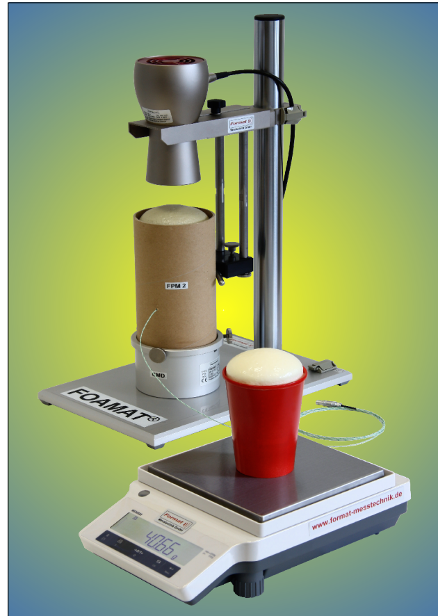
Figure 5: The loss of weight is measured by a laboratory balance integrated into the FOAMAT system. The foam residue remaining in the mixing cup is used for this purpose.
