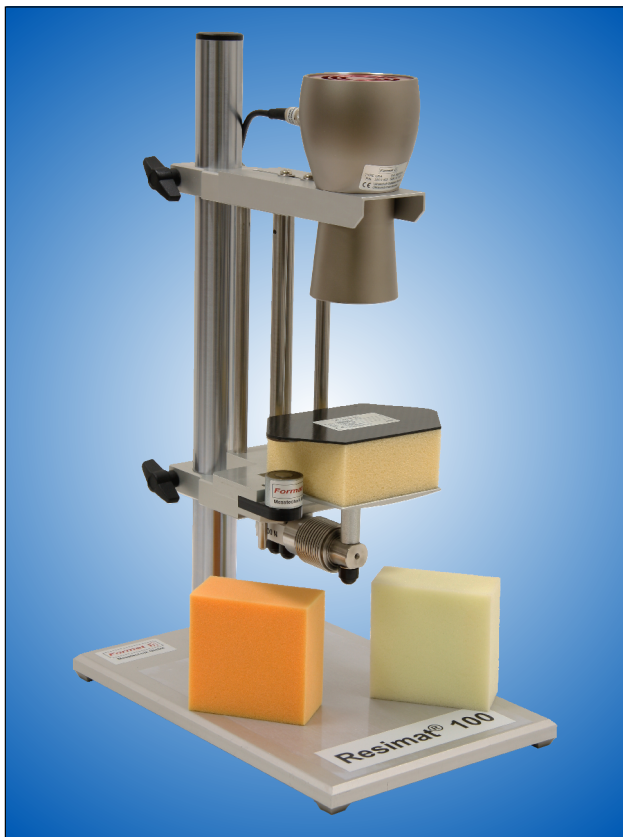
Figure 21: Mechanical setup of Resimat 100 of the product generation 287 for measuring viscoelastic foam samples with typical dimensions of 100x100x50mm 3 .
