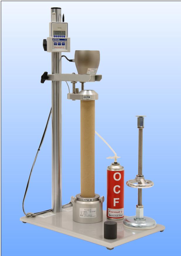
Figure 10: The One Component Foam Measurement device OCFM has a special holder for aligning the FPM 50 and the cardboard cylinder under the ultrasonic sensor. The Perfect Preparation Aid PPA (right) helps to inject a defined amount of froth.
