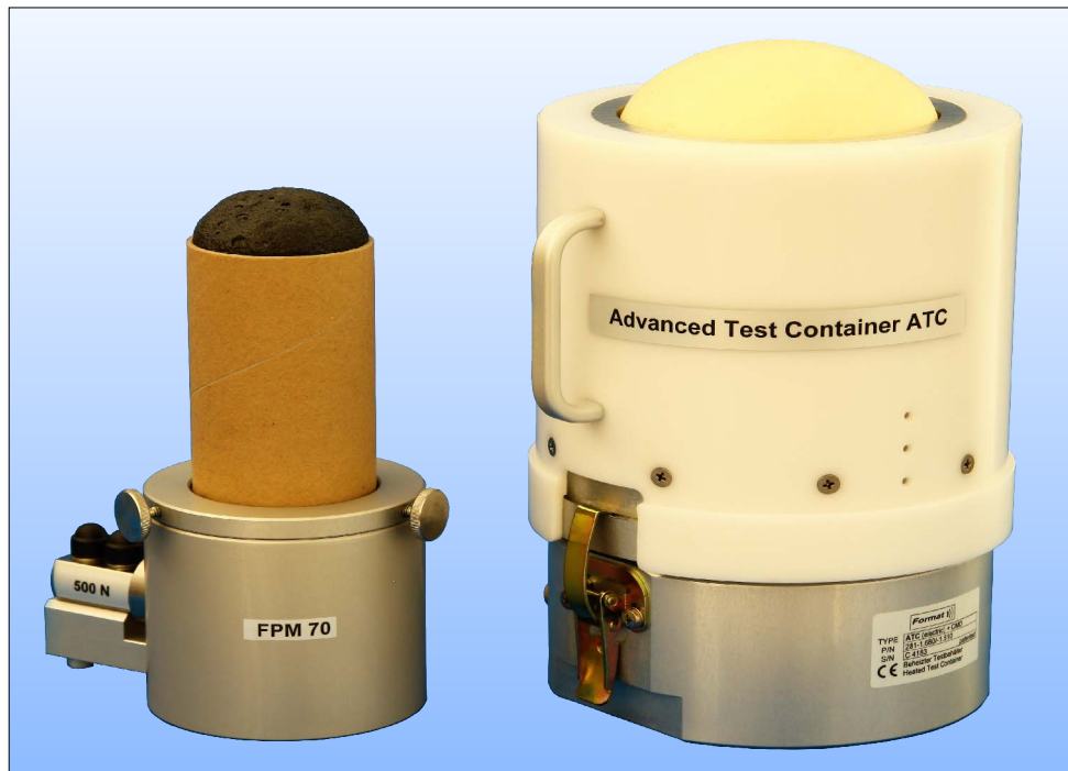
Figure 6: Size comparison of two FOAMAT test containers: The FPM 70 (left) is designed for rise height and pressure measurement of high density foam samples. The picture shows a sealing foam in a 70mm cardboard cylinder. The Advanced Test Container ATC (right) is heatable from the bottom to the top and has semi-cylindrical side walls. The lower part contains an FPM/CMD 150 device for pressure and polarization measurement. The insulated upper part can be lifted to ease the ejection of the cured foam sample.
