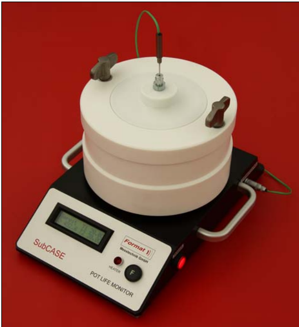
Figure 13: The Test device SubCASE HT can measure the pot life and the curing of reactive plastics. It is designed for high reaction temperatures. The core temperature is measured by a reusable thermocouple inserted vertically into the center of the plastic sample.
