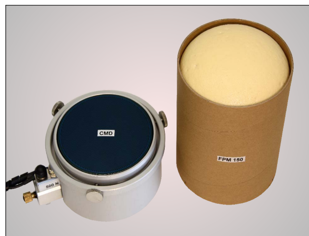
Figure 3: The cardboard cylinder (right) with the cured foam sample can be removed from the Foam Pressure Measurement device FPM 150. The CMD (Curing Monitor Device) sensor is mounted on top of the FPM 150 pressure plate (left). It enables the simultaneous measurement of the dielectric polarization and the rise pressure.
